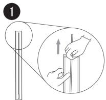
Wear lab globes to prevent contamination and take out the long stem swab carefully so as to not to touch the parts as this may affect the cleanliness level
