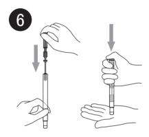
Return the sampling stick to the main body (casing) and push it all the way into the main body.
