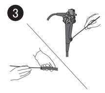
Handle the long stem swab with care so as to not to touch the parts as this may affect the cleanliness level. Insert the long stem swab in the canalicular object to be tested, and wipe it off as long as the length of the long stem swab reaches, and pull the swab up slowly.
