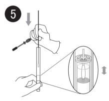
Insert the long stem swab in the main body(casing) of the LuciPac Pen-AQUA to push and break the center of the upper seal of the container. Be careful not to break bottom seal of the container for releasing reagent. Remove the long stem swab after thoroughly washing the cotton bud in the releasing reagent.
