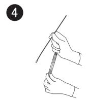
Hold the long stem swab at 12 cm or 13 cm distant point from the cotton bud, and remove the sampling stick from the main body (casing) of the LuciPac Pen-AQUA by your free fingers. Handle the sampling stick with care so as to not to touch the parts as this may affect the cleanliness level.
