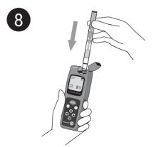
Insert the LuciPac Pen-AQUA into the Lumitester and close the Lumitester measurement chamber cover.
